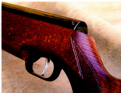
Picture shows same Blade from a different angle with RS Safety Catch in fire mode.
